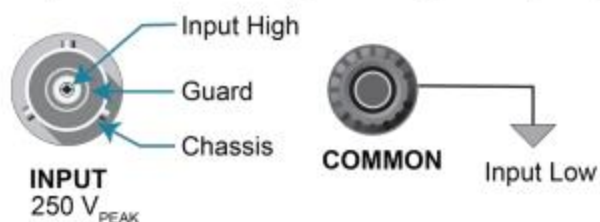
Figure 9: Input connector configuration - guarded (voltage only)
