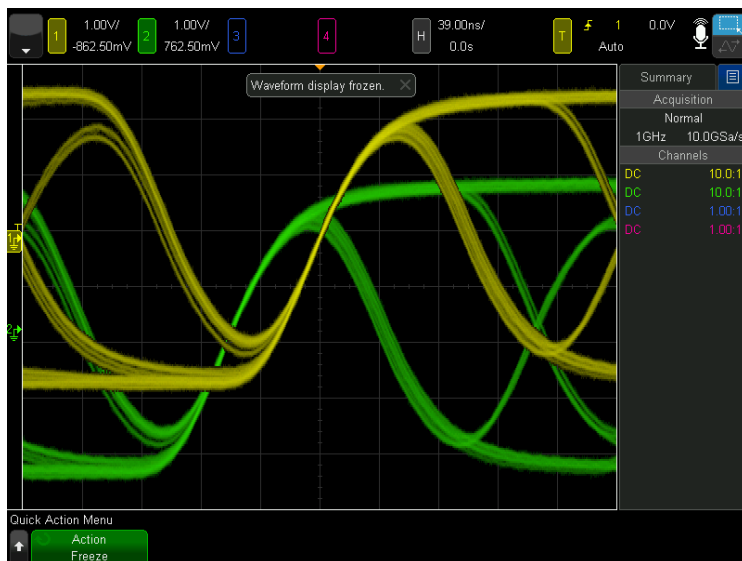
Figure 54. Quick Freeze Display preserves the persistence.
